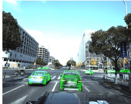
Figure 1: 6D-VNet is trained end-to-end to estimate vehicles’ six degree of freedom poses from a single monocular image. The output will precisely estimates the vehicle’s voxels in 3D occupancy.
